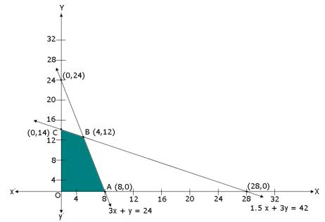
The corner points are A(8,0), B(4,12), C(0,14) and O(0,0). The values of Z at these corner points are tabulated as follows:
